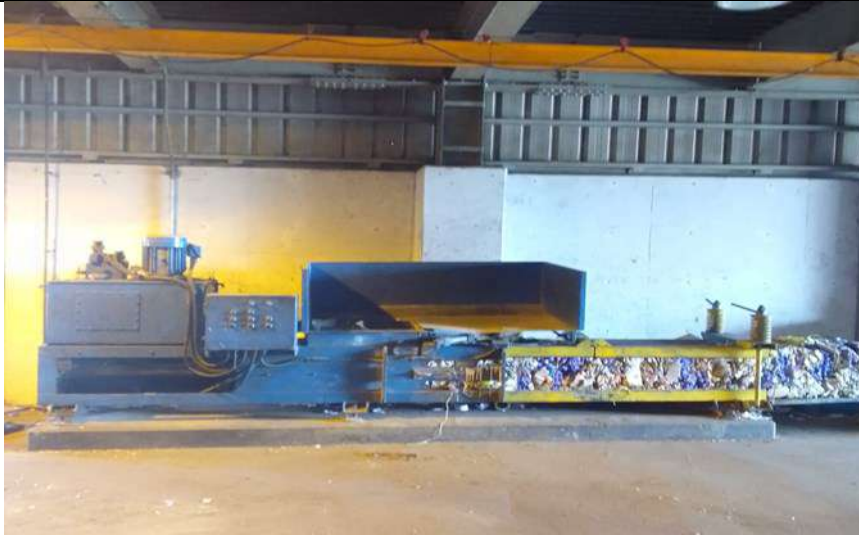
Paper and carton baler in Nahdet Misr company for wastes collection in Alexandria
