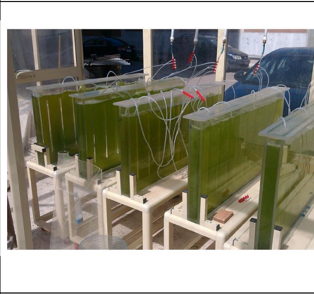
Algae Cultivated In Flat Panel Photo-Bioreactor, Med-Algae Project (Faculty of Science, Alexandria University)
