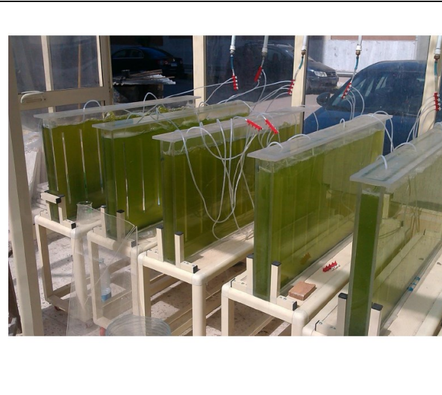
Algae Cultivated in Flat Panel Photo-Bioreactor, Med-Algae Project (Faculty of Science, Alexandria University)
