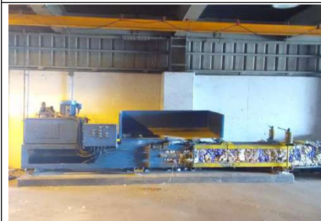
Paper and carton baler in Nahdet Misr company for wastes collection in Alexandria
