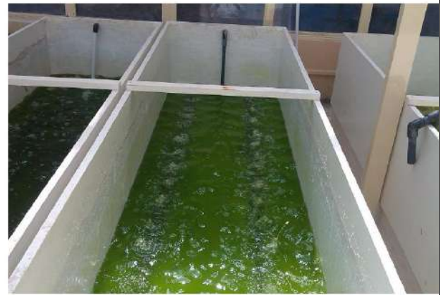
Open Ponds with running algal cultures, Med-Algae Project (Faculty of Science, Alexandria University)
