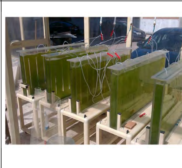
Algae Cultivated In Flat Panel Photo-Bioreactor, Med-Algae Project (Faculty of Science, Alexandria University)
