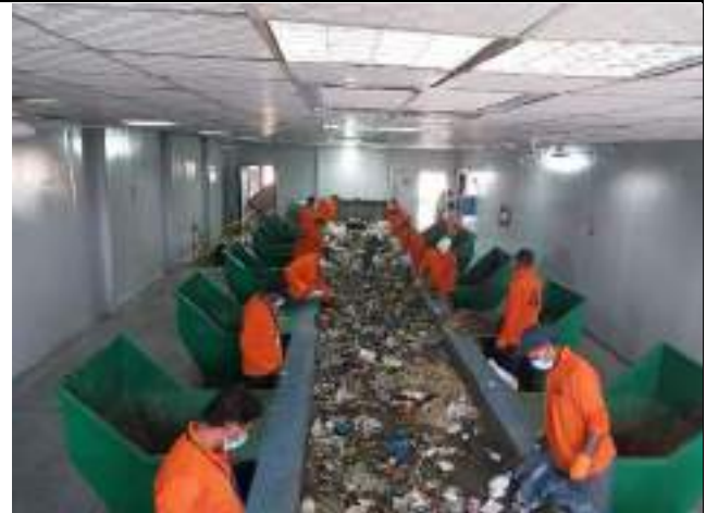
Manual sorting hall in Nahdet Misr company for waste collection in Alexandria
